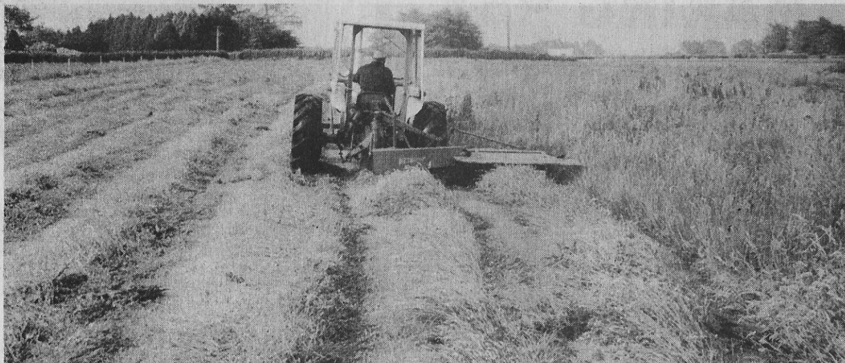
The first step is to cut the hay and today's modern mowers make swift work of it. Most mowers today are of the large disc type (similar to rotary lawn mowers) outmoding the old blade system.
