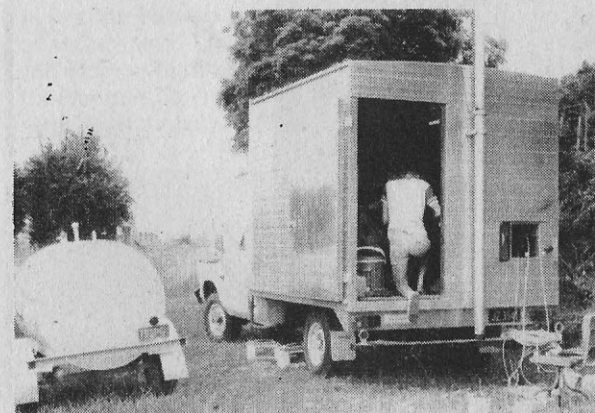
The control base for the operation. It is here that computer equipment records the series of explosions on each section and also records the shock waves of these explosions downwards into the earth's structure. These are recorded on computer tapes and these tapes are later analysed to produce maps for study.
