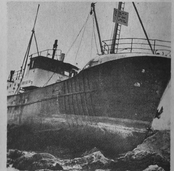
Her plates are bent and buckled and she is wedged tight.
