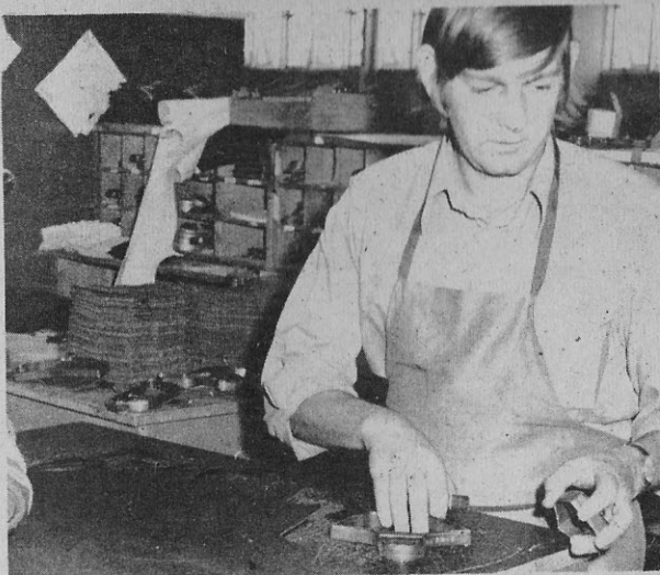
Peter Berge cuts out the shoe from the raw material. The leather is cut into several different sections before being assembled
