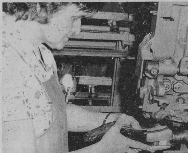
Mrs Helen Tygelski attaches the shank which runs through under the shoe for firmness and support
