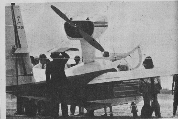
This craft is called a Lake Buccaneer and is rather eye-catching as the propeller is mounted above the fuselage, facing to the rear
