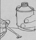
6. Paint the metal edges of the hole or treat with an anti-rust compound before applying the paint.
