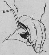
1. Select a point about one-third of the way back along the mudguard. Get someone to hold the mirror there while you sit in the driving seat to make sure you can see the mirror without having to crane past a wind screen pillar.
