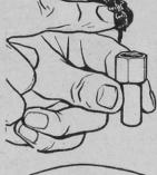
7. If the mirrors are of the flyback type, fill the plastic cups with thick grease before the final assembly. This will prevent any seepage of rainwater in service and also help the flyback action.
