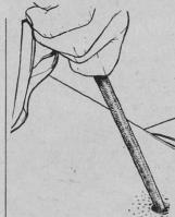
5. File the hole to a perfect roundness and check with the mirror stem at frequent inter-vals. Don't use a file so large that it will stick in the hole, and hold it at an angle to the surface while you're filing. Don't be in too big a hurry or the file may pull right out and scratch the paint.
