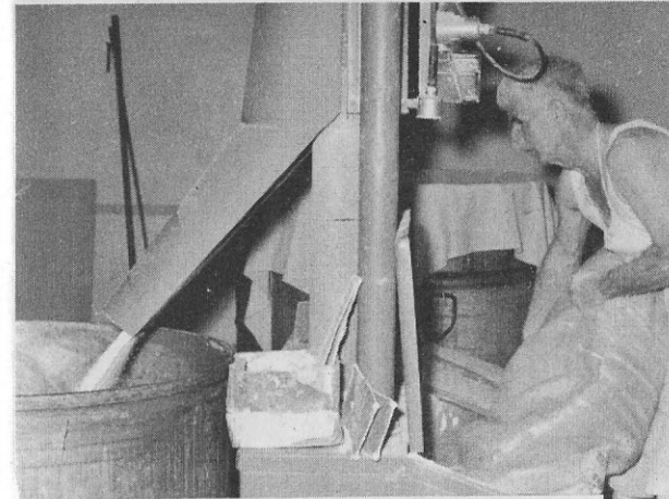
Bert Goldfinch lifts the flour into the sifter, which takes out all impurities.
