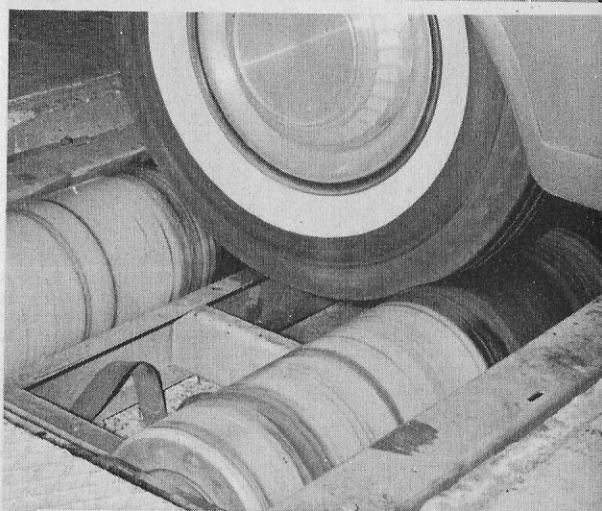
Loaded rollers simulate a load on the engine
