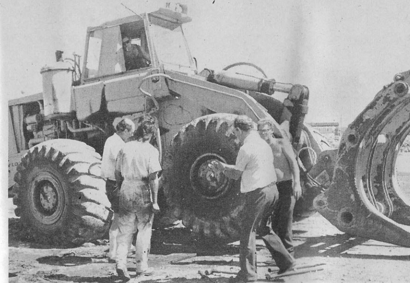
The machine uses its own hydraulics system to lift the front off the ground for the tyre changing
