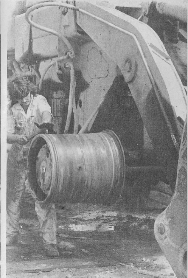
After removal the hub has to be cleaned with a wire brush and then greased before the new tyre is fitted. Here John Wray gets busy with the wire brush
